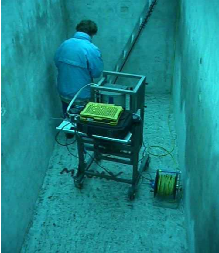
Control measurements by in-situ gamma spectrometry
